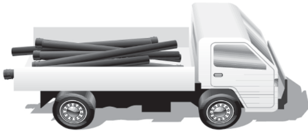
Incorrect way to load pipes
