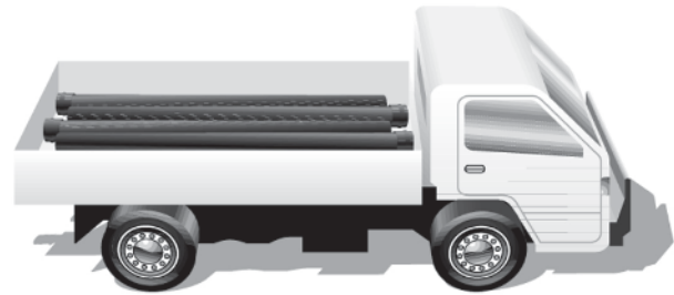
Correct way to load pipes
