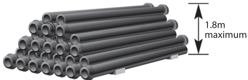
Individual pipe stacks on site
