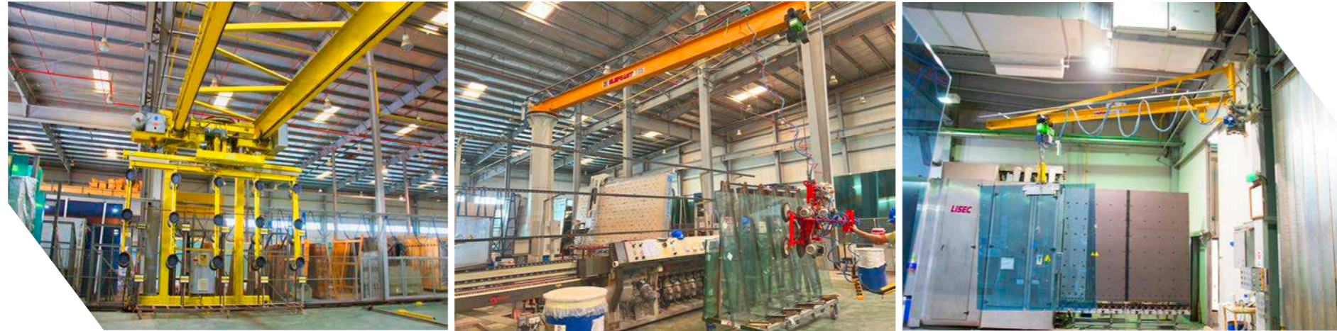
Left: Auto Loading Gantry PKL, Middle: Polishing Line Jib Cranes Lifting System, Right: Double Glazing Line Over Head Clamp Lifting System
