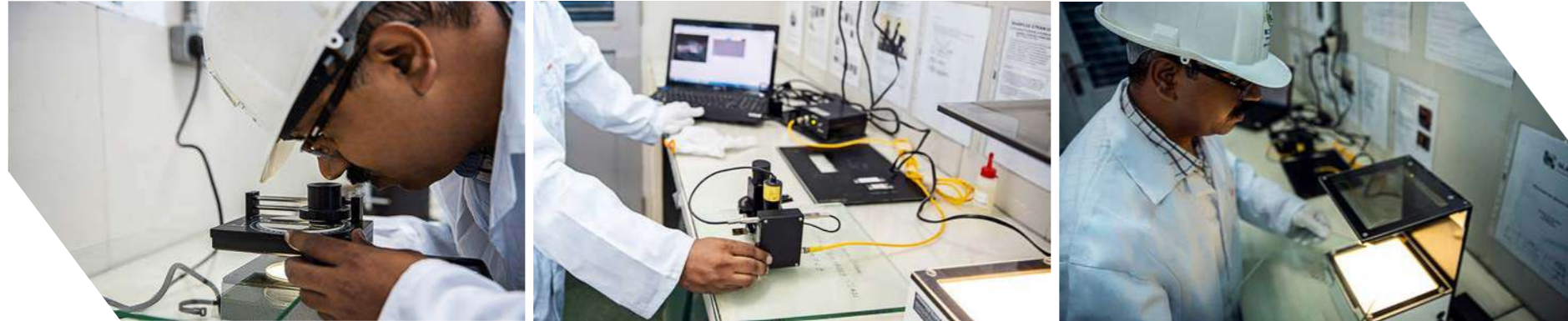
Left: Measuring Edge Stress, Middle: Measuring Surface Stress (GASP), Right: Coating Test
