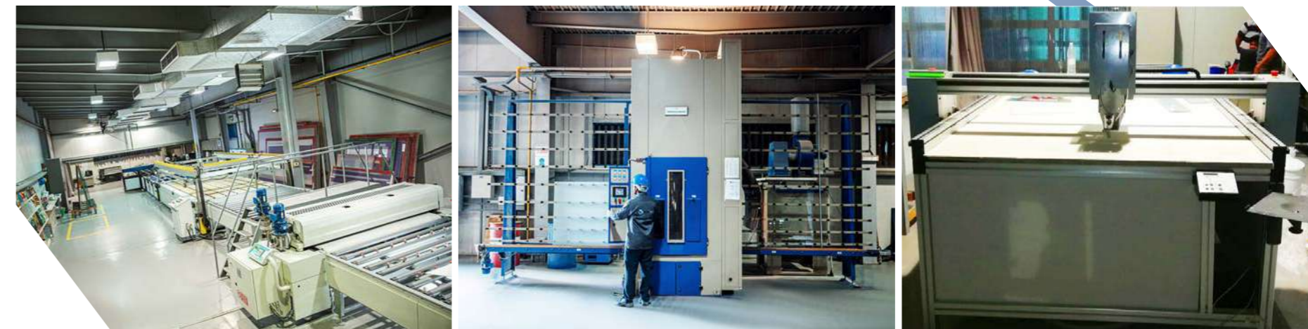
Left: Ceramic Fritting Silk Screen Printing Machine, Middle: Sandblasting Machine, Right: Resin Machine
