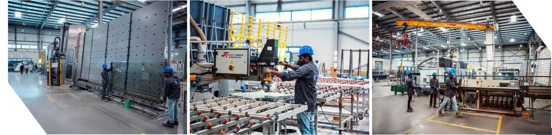
Left: Glass Washing and Grinding (KSR), Middle: Drilling Unit, Right: Single Edger Machine
