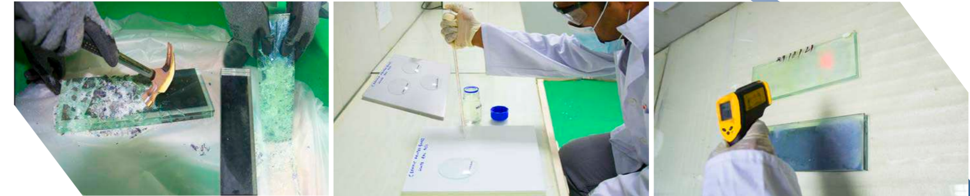
Left: Pummel Test, Middle: Acid Resistance of Ceramic Decoration on Architectural Glass, Right: Digital Condesspot Pro temp and Humity Tester
