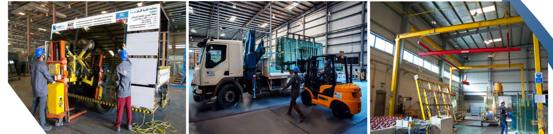
Left: Glass Loading Unit, Middle: Forklift, Right: Lamination Line Over Head Clamp Lifting System
