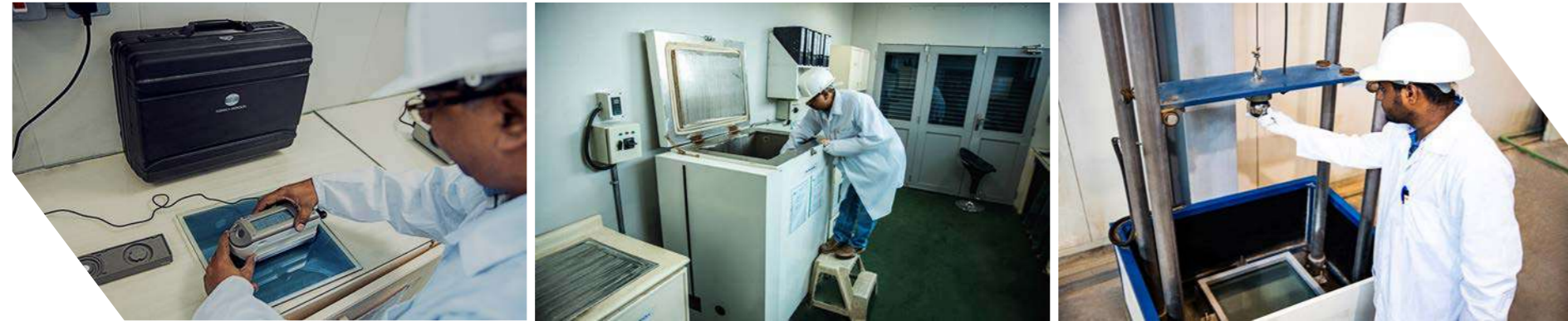
Left: , Middle: Low e Glass Emissivity Measurement, Right: Ball Drop Impact Resistance Test of Laminated Architectural Flat Glass
