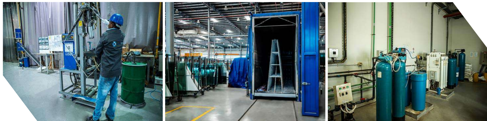
Left: Desiccant Filling Machine, Middle: Heat Soak Testing Unit, Right: Reverse Osmosis Demineralization
