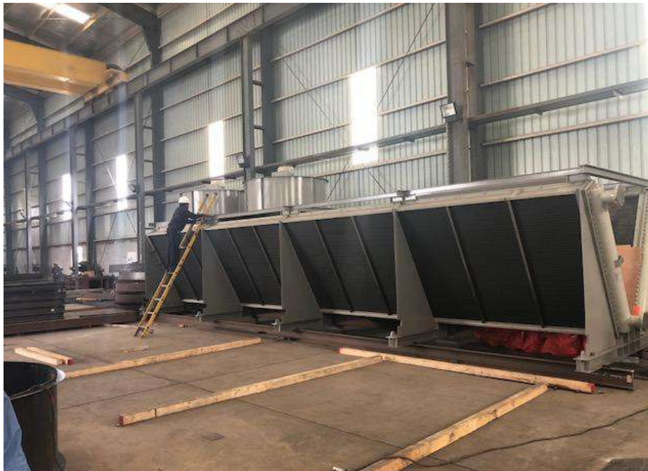
Fabrication & Assembly of Fin Fan Cooler modules & structure for B&W SPIG (GE-GAMA Power for Alba PS-5 Project)
