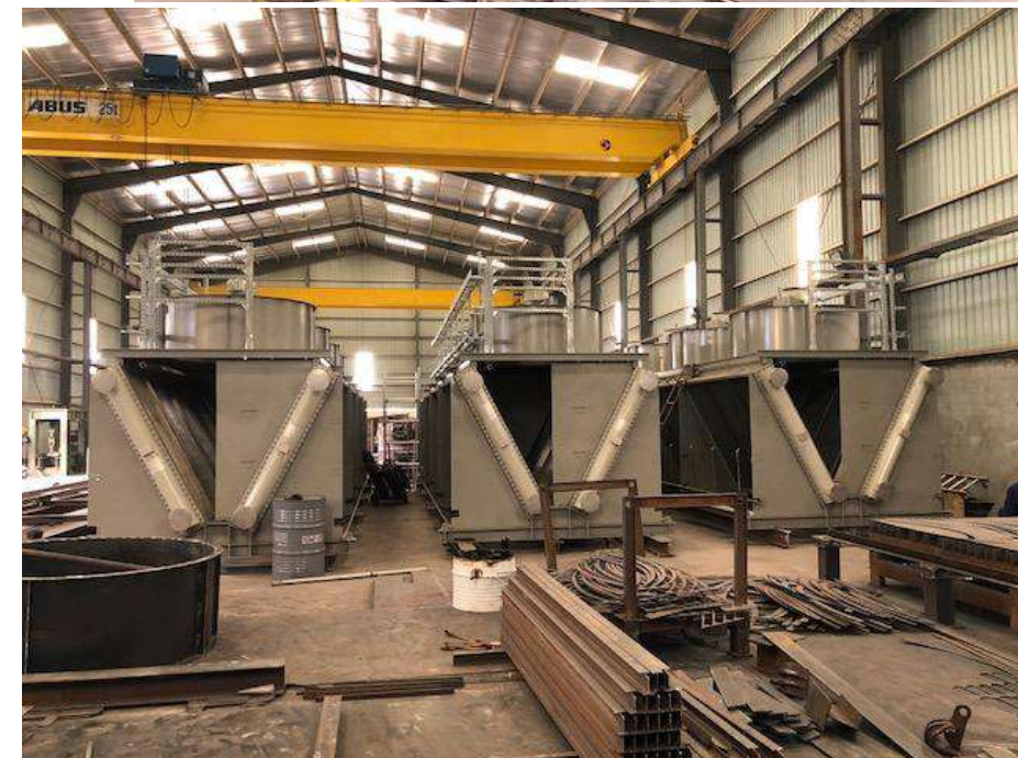
Fabrication & Assembly of Fin Fan Cooler modules & structure for B&W SPIG (GE-GAMA Power for Alba PS-5 Project)
