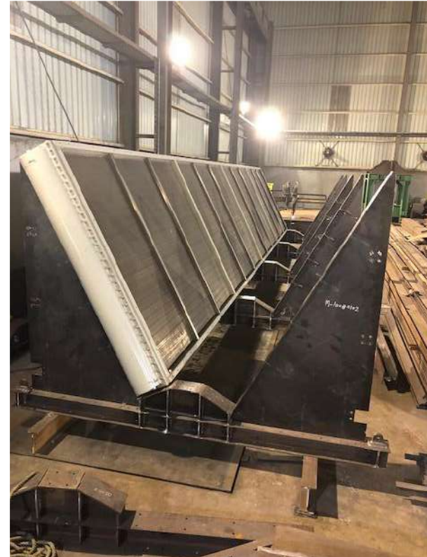
Fabrication & Assembly of Fin Fan Cooler modules & structure for B&W SPIG (GE-GAMA Power for Alba PS-5 Project)
