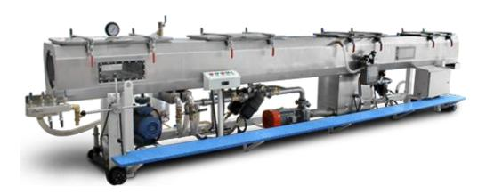
Are used for calibrating and cooling pipes made of thermoplastic materials by means of spray cooling. The spray cooling method prevents the formation of water boundary layers and is more efficient in cooling than the full water tanks.
