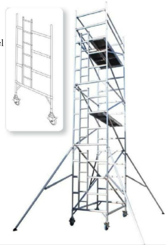
ALUMINIUM DW SCAFFOLDING 1.45 M WIDTH X 2.5 M LENGTH LOAD CAPACITY: 250 KG PER PLATFORM | 750 KG PER TOWER
